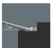
The ring side is cranked at 15° to the tool axis to prevent injury.
